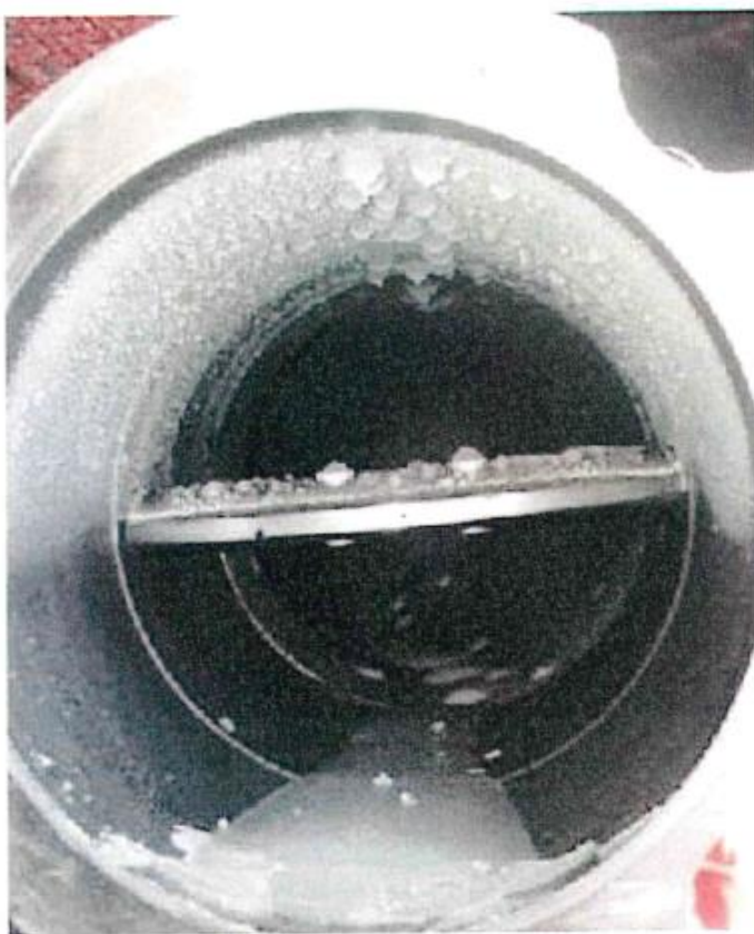
Figure 1, Ice Obstruction in Engine Intake Throttle Actuator
